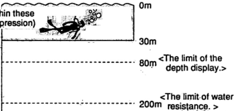
**b. The water depth meter in this watch is set according to the sea water standard (1.025 gravity).**
