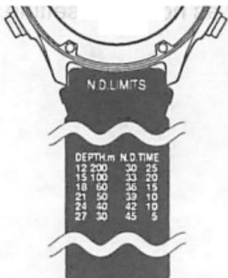
When a diver has completed a dive, and is ascending to the surface, the speed at which a diver can ascend to the surface, without stopping for decompression, is decided according to the diving depth and diving time. These limits are marked as no decompression limits. The no decompression limits which are on the watch band, are based on the US navy diving manual (1985 edition).
